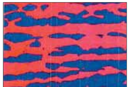
Figure 4 – Phase distribution at 500x magnification
